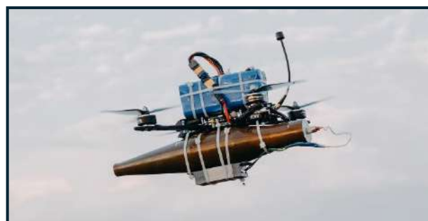
Figure 5: An FPV Kamikaze drone equipped with an improvised explosive payload
