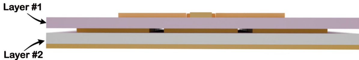
Figure 27: Multilayer patch antenna, with two different substrates. Source: Sara Reiss et al 67
