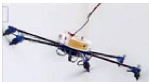
Figure 2: Forward Advancing Tilt-Hex platform with six unidirectional propellers. Source: Mengtang Li 12
