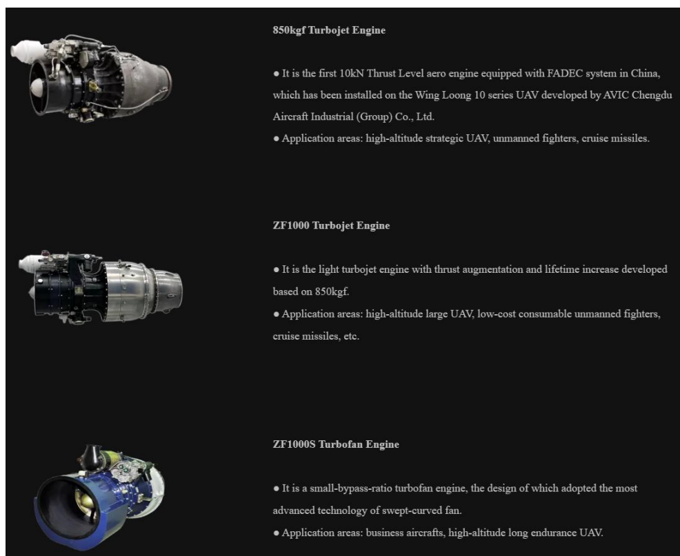
Figure 20: Chinese Drones Engines Options (Source- Sino-Defence Forum 48 )
