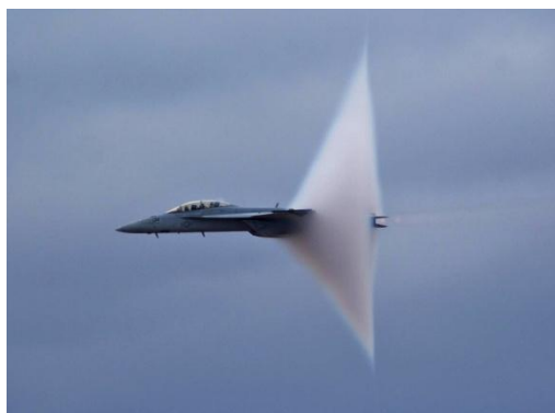
(Fig.13 An aircraft with a visible shockwave developed)
