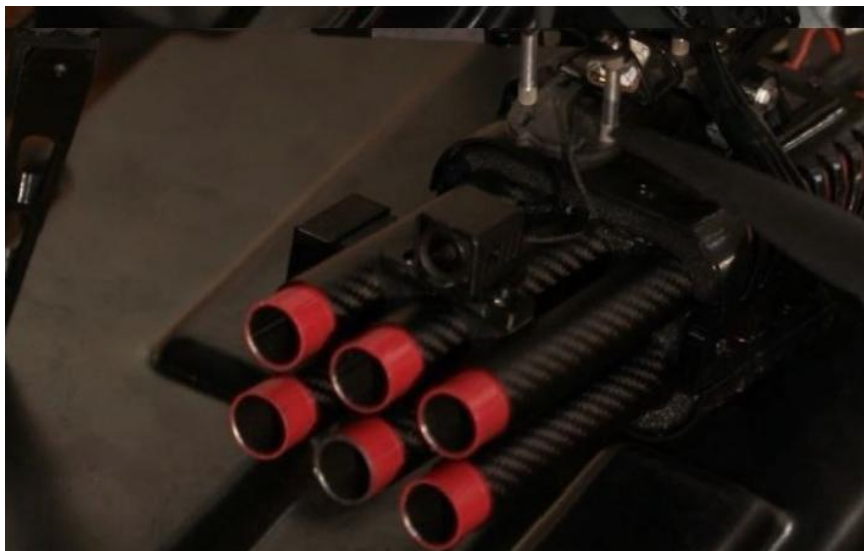
Figure 3: 6 Barrel Shotgun FPV Drone
