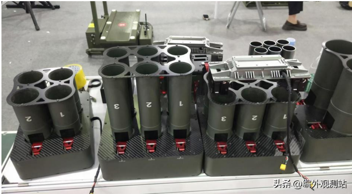
Figure 2: Drone Mounts for Mounting Munitions (Source- Chinese Website Toutiao 45 )
