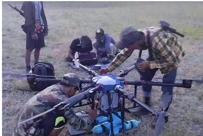
Figure 11: Preparation of a Hexacopter for Mortar Rounds' Bombing Strike (Source-NetEase 85 )
