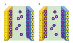
(Schematic diagram of (a) an electrical double layer capacitor and (b) a pseudo capacitor.)
