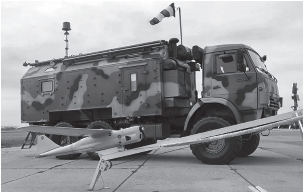
Figure 3 : Russian Leer-3 EW System with Orlan-10 Drone for Range Extension. Source : https://spectrum.ieee.org/the-fall-and-rise-of-russian-electronic-warfare
