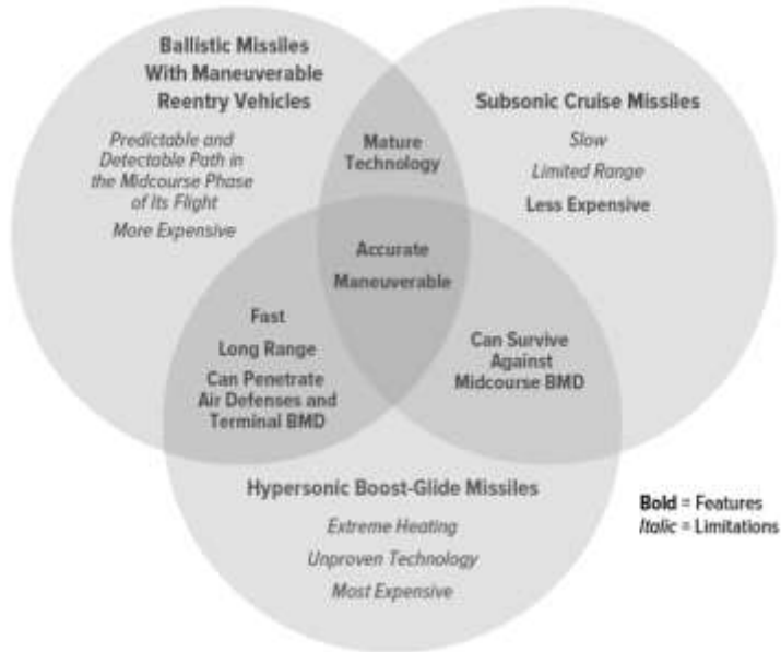
Fig.1: A holistic comparison between ballistic missiles, subsonic cruise missiles and hypersonic boost glide (Source :- U.S. Congressional Budget Office ( https://www.cbo.gov/publication/58924 ))
