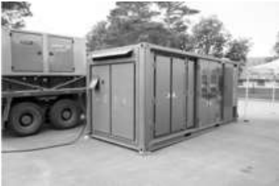
Fig – 5, Field Deployable 3D Printing Source: UK MOD Army, “British Army Deploys 3D Printing in the Field”, 10 May 2024 https://www.army.mod.uk/news-and-events/news/2024/05/brokkr-pioneering-the-british-army-s-deployable-additive-manufacturing-capability/ .
