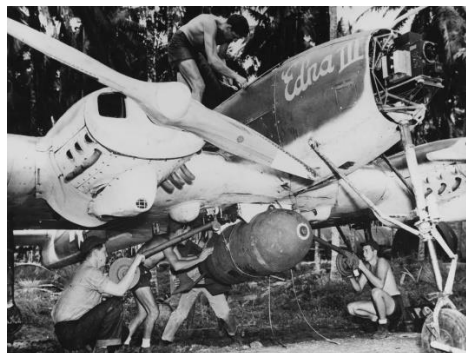
(A TDR-1 being prepared for a mission on Mbanika Island, in the Solomons. Note the TV camera in the nose.)
