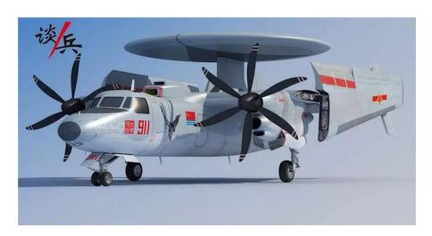
8. Judging from the images, the KJ-600 has a very tight fuselage design, making it almost as long as the J-15 aircraft carrier-based fighter jet, and the Z-18 early warning helicopter. The aircraft carries a radar on the top of its fuselage, similar to China's previous early warning aircraft KJ-2000 and KJ-500. It uses two WJ-6C turboprop engines, but could switch to the newer WJ-10s in the future.
