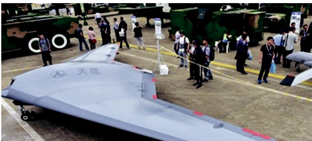
Figure 1 – Sky Hawk (Tian Ying) MUM-T Capable HALE UAV (Source: South China Morning Post)
