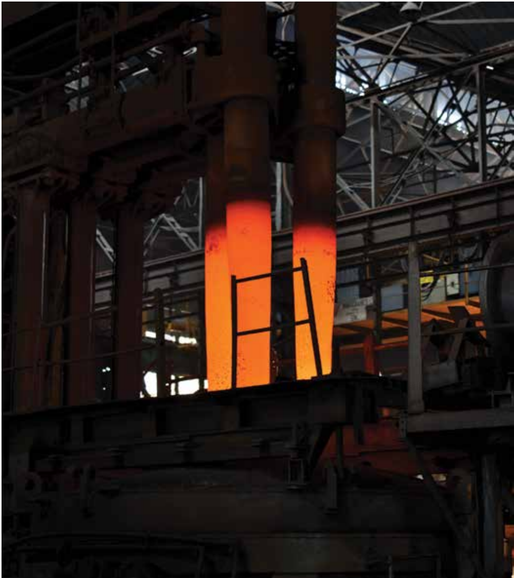
Forging and Manufacture of 155mm 45 Calibre Dhanush Gun Barrel in Metal & Steel Factory of OFB
